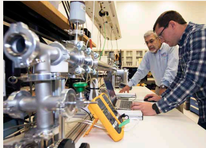
Dr. Carlos Calle, lead scientist in Kennedy Space Center's Electrostatics and Surface Physics Laboratory, left, and Jay Phillips, a research physicist, are modifying an electrostatic precipitator. On Mars, the device would allow astronauts to extract useful elements such as oxygen, water and methane. Photo credit: NASA/Kim Shiflett
