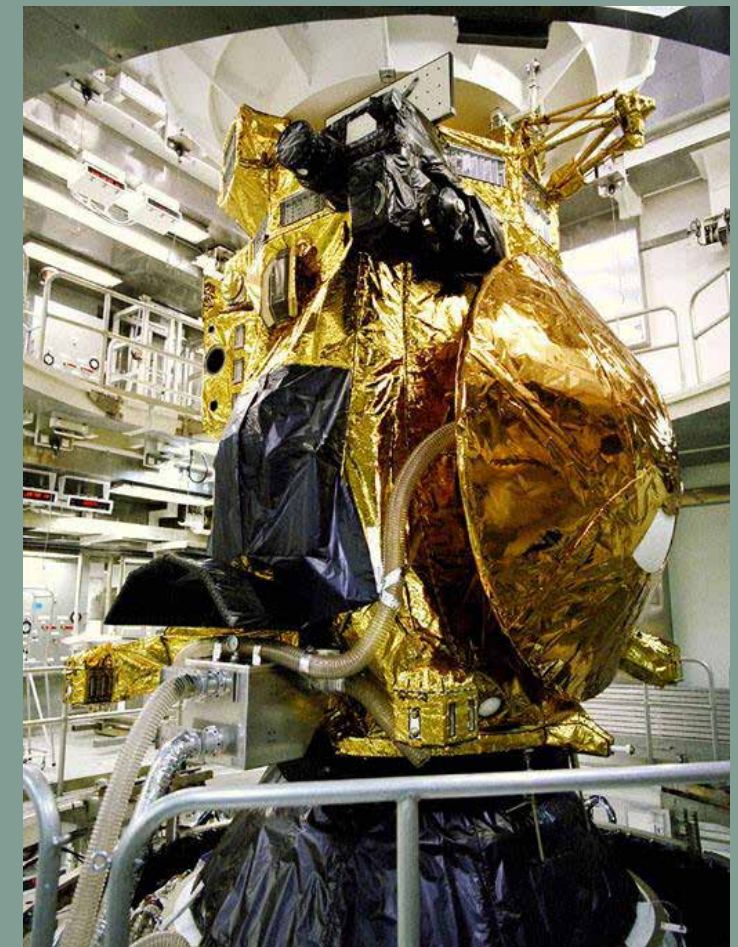
The Cassini spacecraft, with the Huygens probe, sits atop a Titan IVB expendable launch vehicle at Launch Complex 40 at Cape Canaveral Air Force Station on Sept. 21, 1997, where it awaits placement of its payload fairing to protect Cassini during launch. Instruments mounted on the Huygens probe were developed by the European Space Agency. Photo credit: NASA
