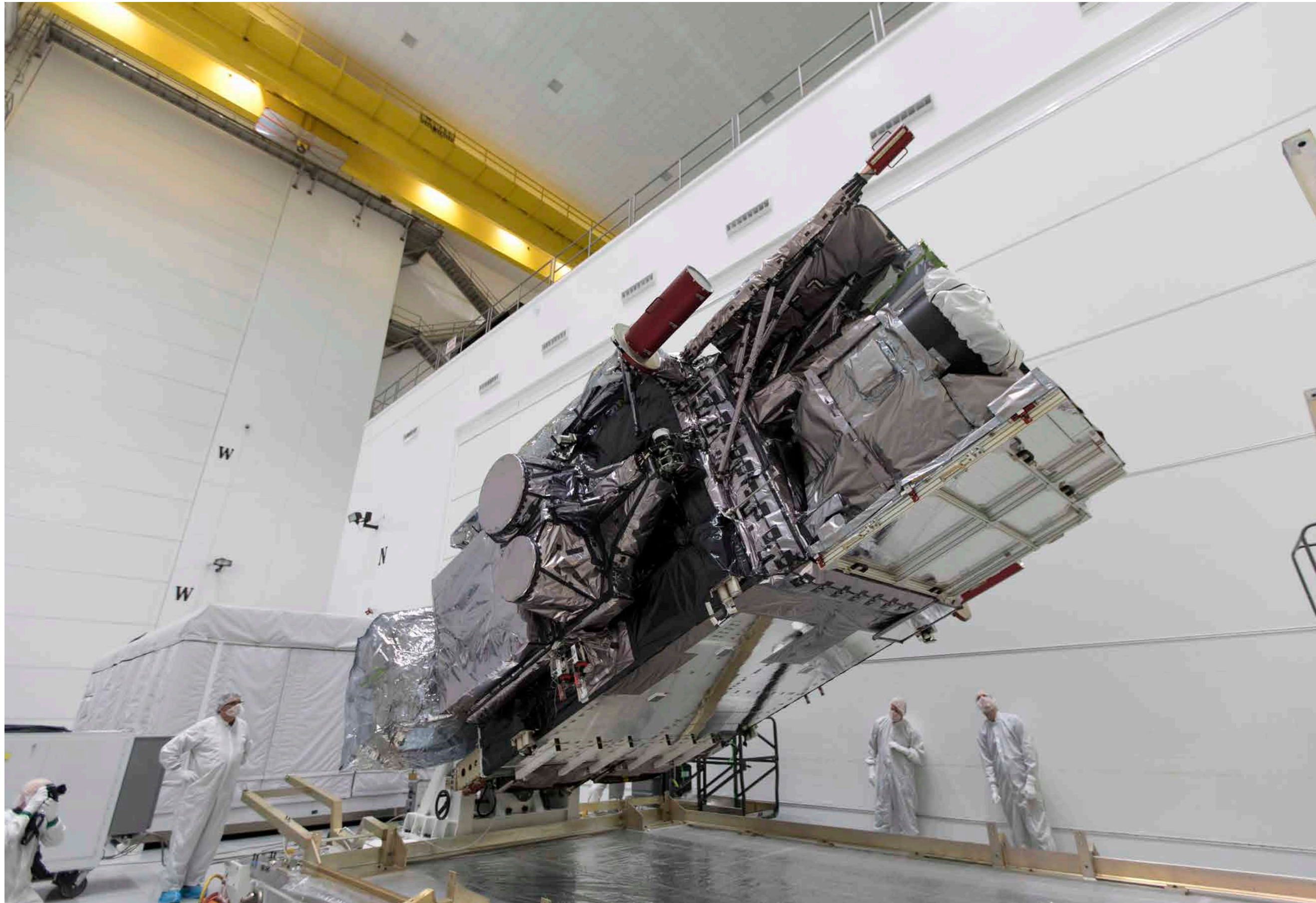
NOAA's Geostationary Operational Environmental Satellite-S, or GOES-S, is rotated from horizontal to vertical for the start of prelaunch processing activities at Astrotech Space Operations in Titusville, Florida, near Kennedy. GOES-S is the second in a series of four advanced geostationary weather satellites. It is slated to launch March 1 aboard a United Launch Alliance Atlas V rocket from Cape Canaveral Air Force Station. Photo credit: NASA/Kim Shiflett
