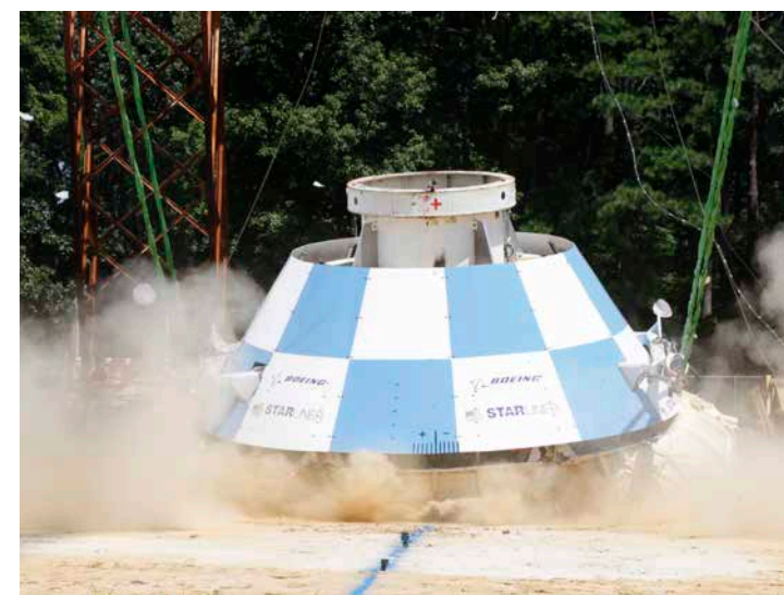
The Boeing Starliner program has performed more than 20 landing tests to determine how the vehicle would fare on land. Photo credit: NASA/Dave Bowman
