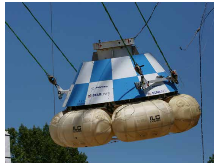
The Boeing Starliner spacecraft undergoes testing at the Landing and Impact Research Facility at NASA's Langley Research Center. Photo credit: NASA/Dave Bowman
