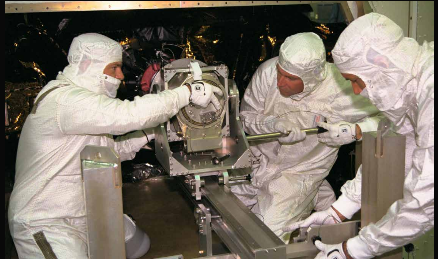
Workers install three radioisotope thermoelectric generators (RTGs) on the Cassini spacecraft Oct. 10, 1997. RTGs are lightweight, compact spacecraft electrical power systems that have flown successfully on previous U.S. missions. These generators produce power by converting heat into electrical energy; the heat is provided by the natural radioactive decay of plutonium-238 dioxide, a non-weapons-grade material. Photo credit: NASA
