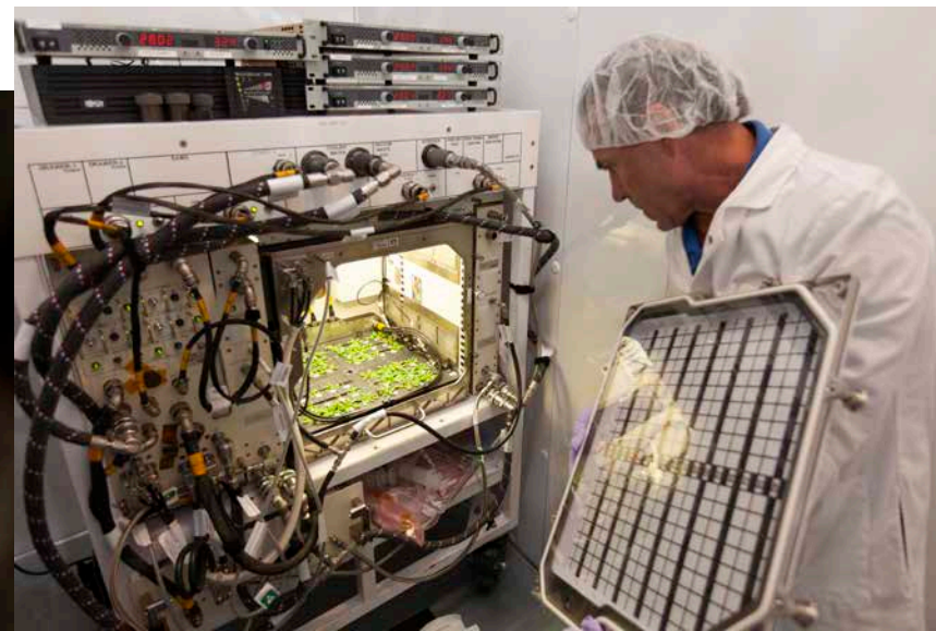
John "JC" Carver, a payload integration engineer with NASA Kennedy Space Center's Test and Operations Support Contract, uses a FluorPen to measure the chlorophyll fluorescence of Arabidopsis thaliana plants inside the growth chamber of the Advanced Plant Habitat Flight Unit No. 1. Half the plants then were harvested. Photo credit: NASA/Leif Heimbold
