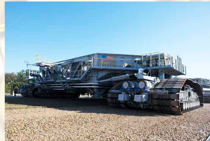
Kennedy Space Center's crawler-transporter is an example of a vehicle with moving parts that require many types of oils and petroleum products available at the Oil Pharmacy. The crawler is the vehicle that will transport the load of the Space Launch System rocket and Orion spacecraft atop the mobile launcher, moving from the Vehicle Assembly Building to Launch Complex 39B. Photo credit: NASA/Leif Heimbald
