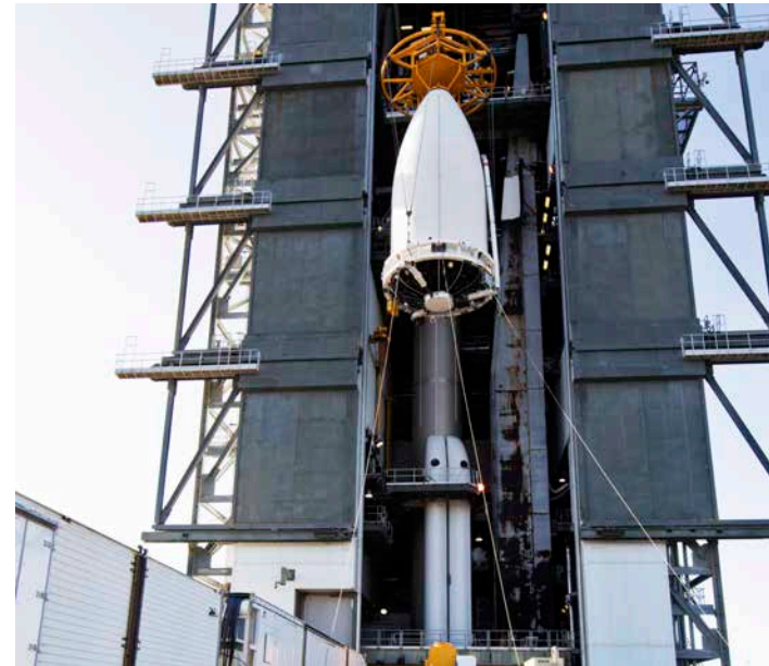
The payload fairing containing NOAA's Geostationary Operational Environmental Satellite-S (GOES-S) is lifted up by crane Feb. 16, 2018, at the United Launch Alliance Vertical Integration Facility at Space Launch Complex 41 at Cape Canaveral Air Force Station. Photo credit: NASA/Glenn Benson
