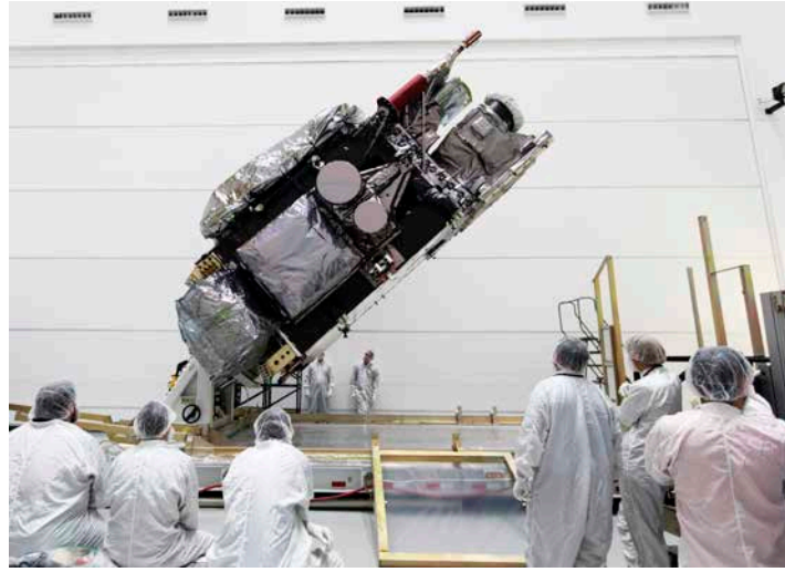
At Astrotech Space Operations in Titusville, Florida, NOAA's Geostationary Operational Environmental Satellite-S (GOES-S), is rotated to a vertical position Dec. 5, 2017, after it was uncrated from its shipping container. The facility is located near NASA's Kennedy Space Center. Photo credit: NASA/Kim Shiflett
