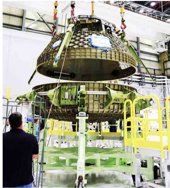
The upper and lower dome sections of a CST-100 Starliner are mated to complete the first hull of the Starliner's structural test article May 2, 2016, in the Commercial Crew and Cargo Processing Facility (C3PF) at NASA's Kennedy Space Center in Florida. The C3PF was Bay 3 of the Orbiter Processing Facility during the space shuttle era. Photo credit: Boeing
