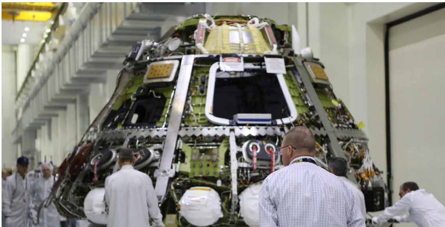
Technicians assist as the Orion crew module for Exploration Mission-1 is moved toward the thermal chamber in the Neil Armstrong Operations and Checkout Building high bay at NASA's Kennedy Space Center in Florida. Photo credit: NASA/Frank Michaux
