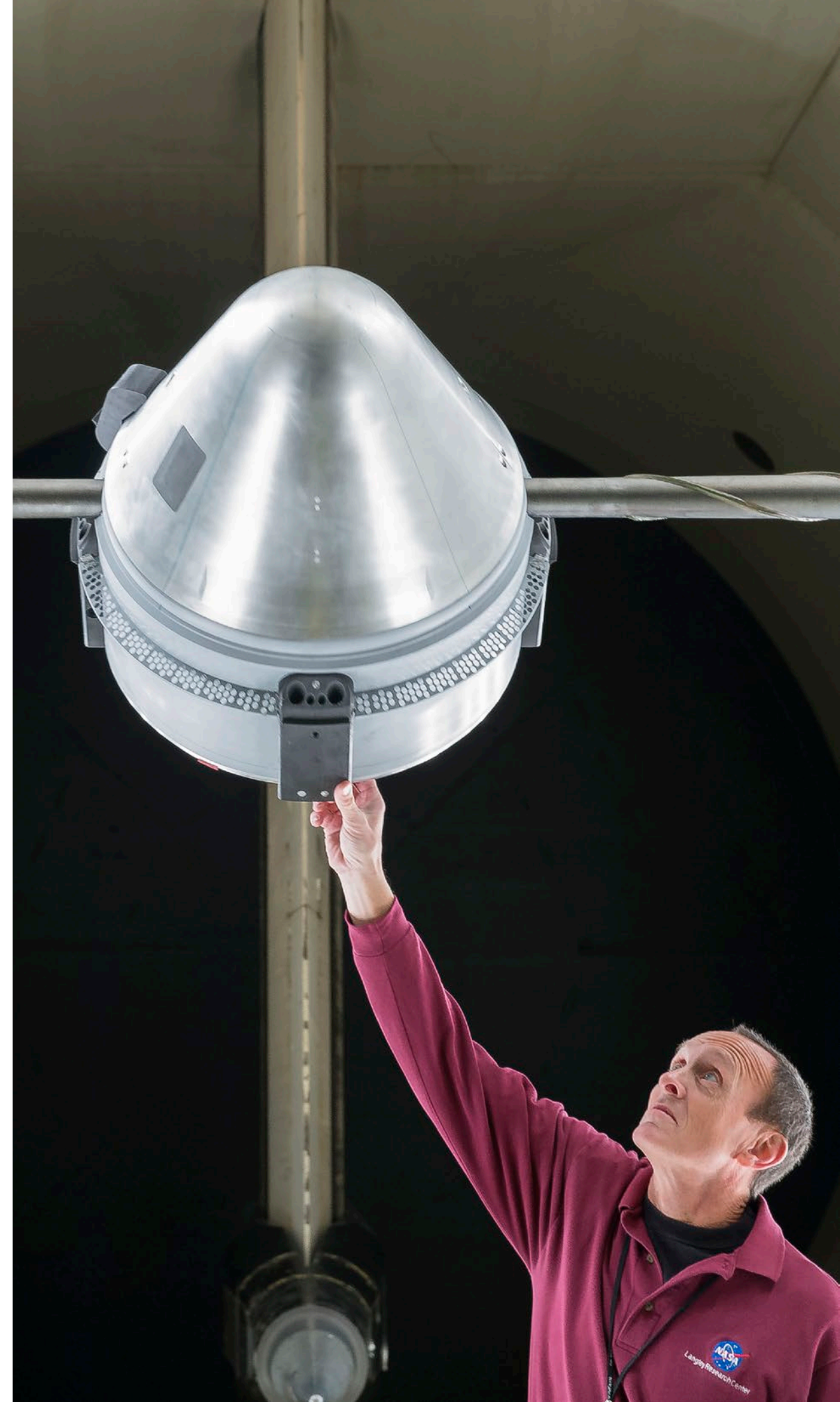
Right: An engineer checks out a scale model of the Boeing CST-100 is set up for evaluation in a wind tunnel at NASA's Langley Research Center in Hampton, Virginia. Photo credit: NASA
