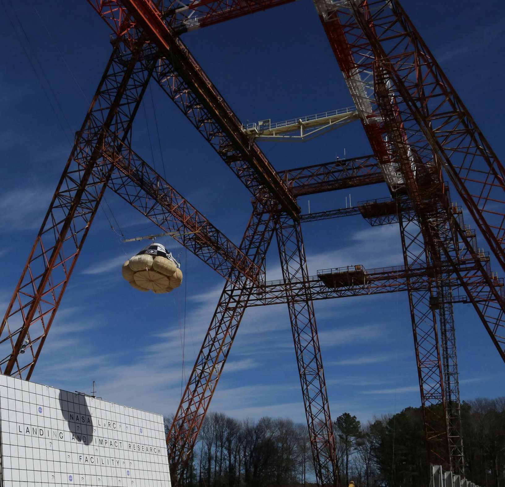
Left: The CST-100 mock up was lifted high into the gantry at Langley to test the water landing characteristics of the design. Photo credit: NASA
