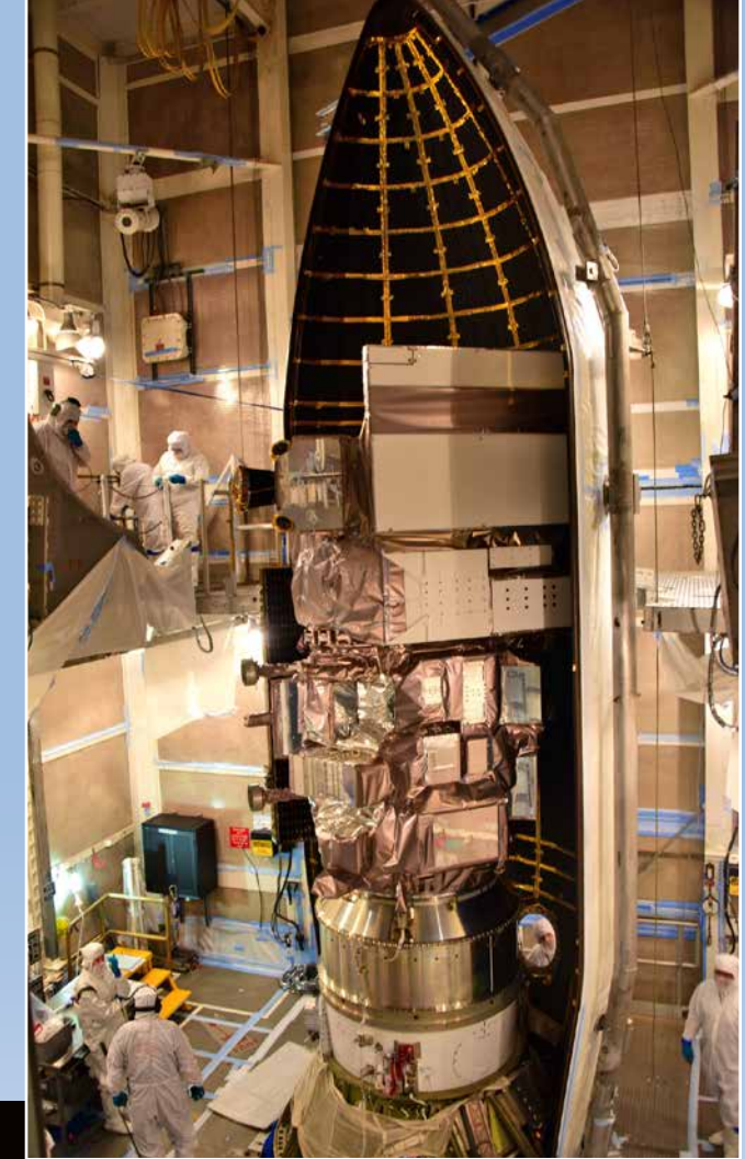
(Right) The first half of the United Launch Alliance Delta II payload fairing is secured around NASA's Ice, Cloud and land Elevation Satellite-2 (ICESat-2) on Sept. 4, 2018, at Space Launch Complex 2 at Vandenberg Air Force Base in California. Photo credit: USAF 30th Space Wing/Alex Valdez
