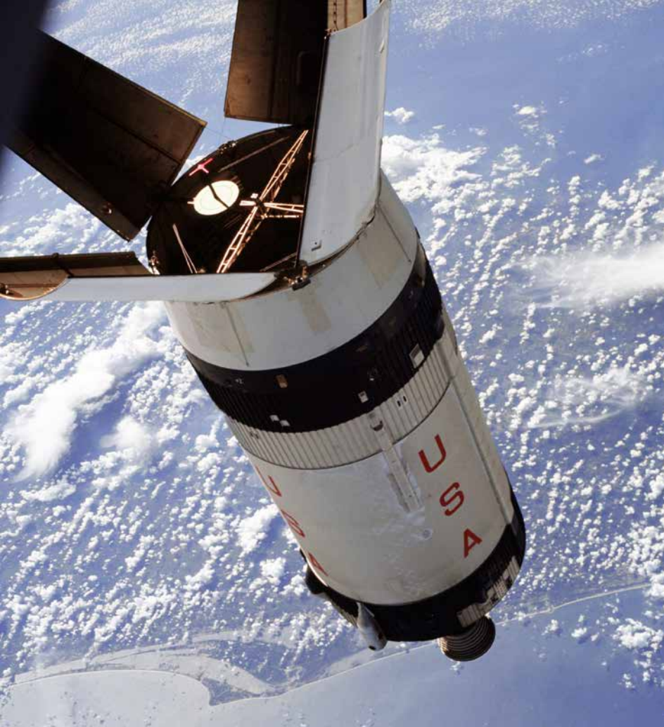
Following launch, the Apollo 7 crew photographed the expended Saturn launch vehicle's second stage, called the S-IVB. NASA's Kennedy Space Center and Cape Kennedy (now Cape Canaveral) Air Force Station are visible on the lower left. The round, white disc inside the open panels of the S-IVB is a simulated docking target similar to that used for docking with a lunar module. Photo credit: NASA
