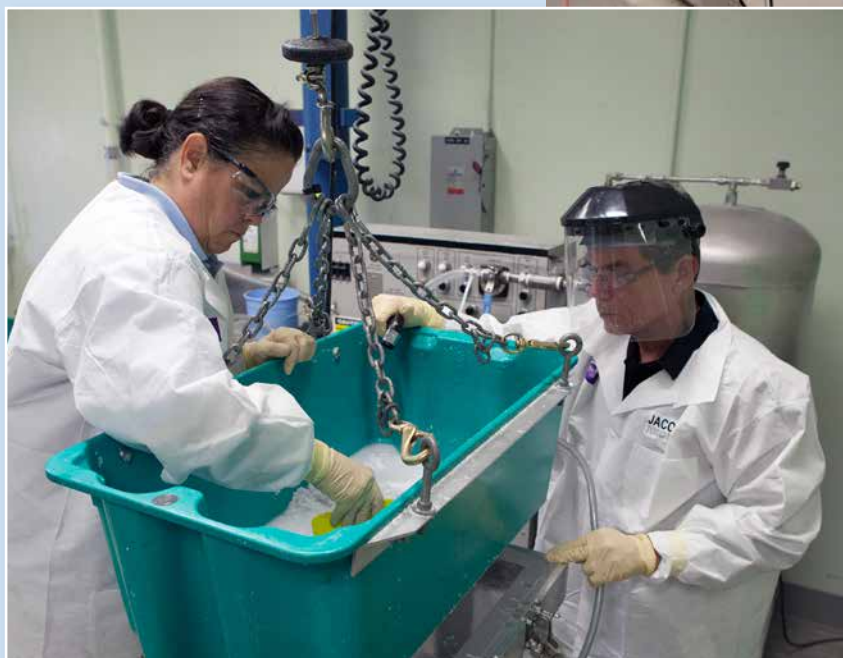
Technicians prepare the slurry used to make a thermal protection system silica-based block in development for Sierra Nevada Corporation's Dream Chaser spacecraft. Photo credit: NASA/Dimitrios Gerondidakis
