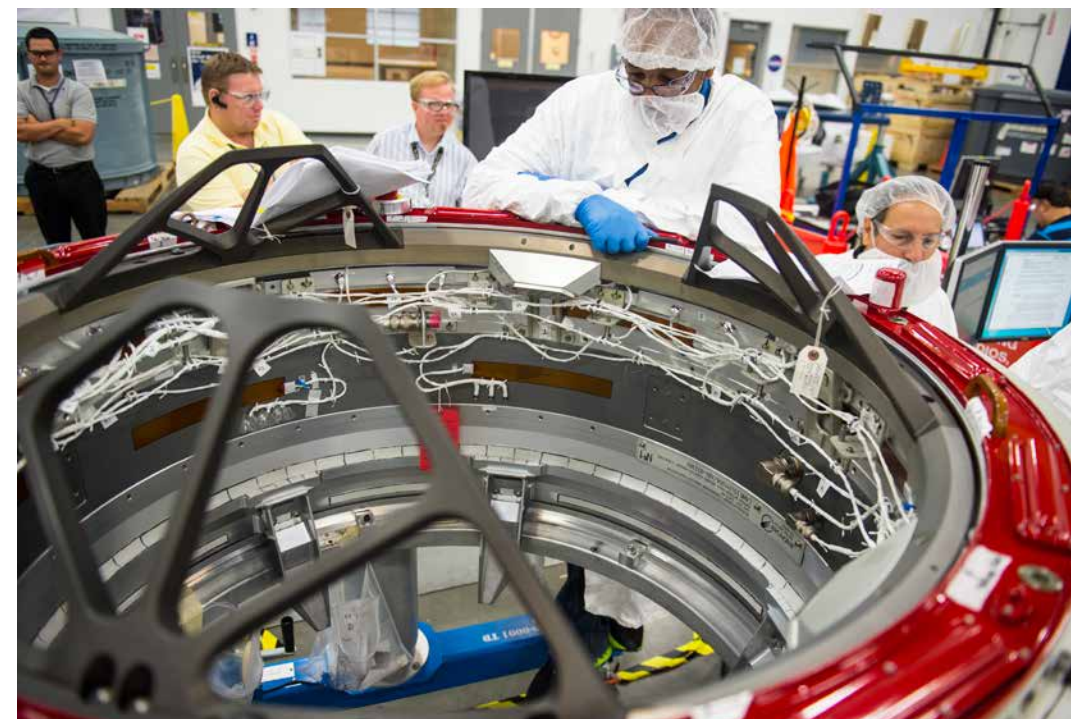
Technicians with The Boeing Co. inspect the International Docking Adapter during its assembly at the company's Houston facility. Photo Credit: The Boeing Co.
