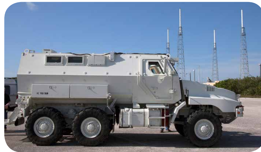
MRAP is a 45,000-pound armored vehicle used to evacuate astronauts and ground operations personnel from danger at the launch pad. Photo credit: Jim Grossmann
