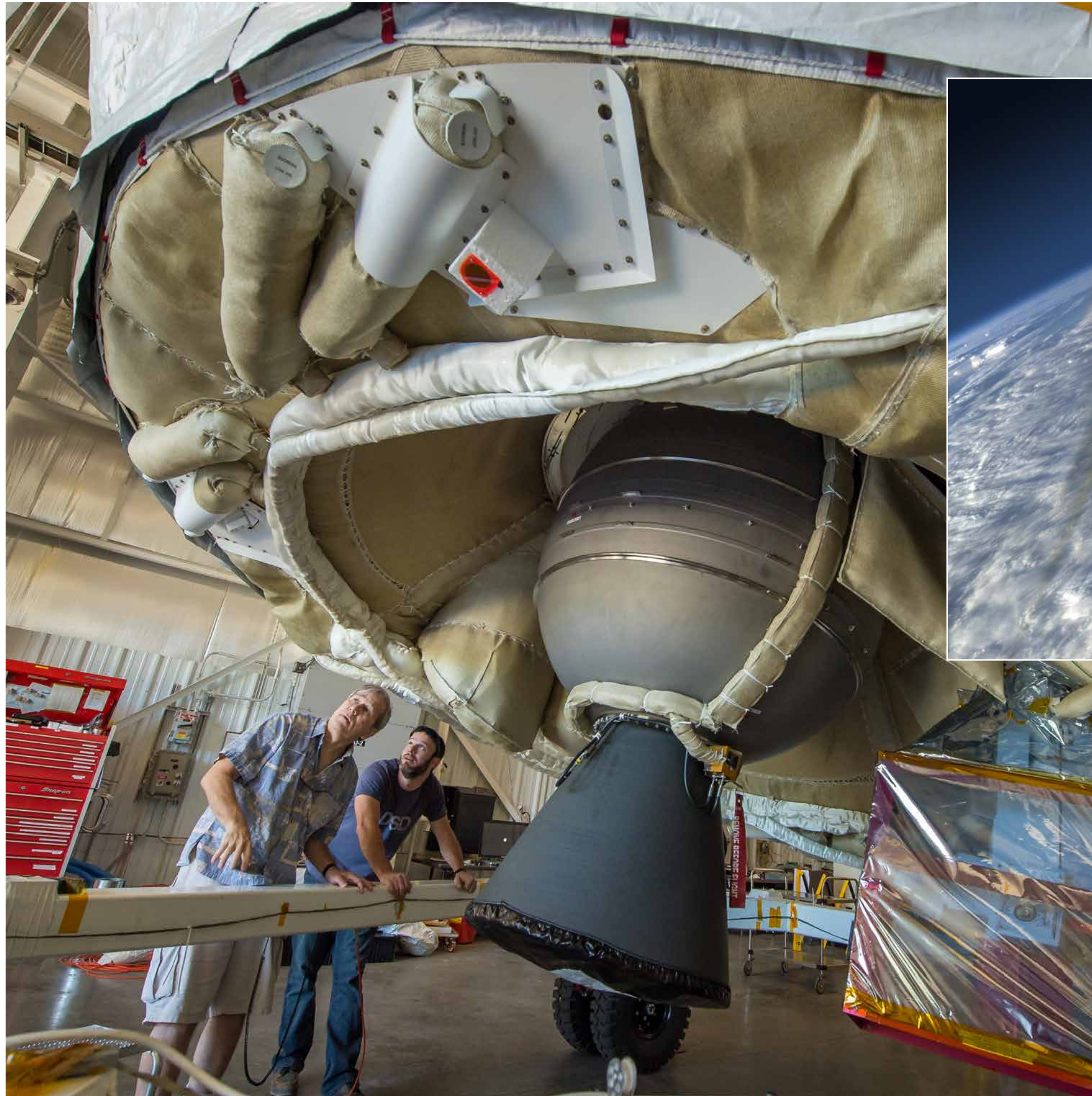
Above: This artist's concept shows the test vehicle for NASA's Low-Density Supersonic Decelerator, designed to test landing technologies for future Mars missions. A balloon lifts the vehicle to high altitudes, where a rocket takes it even higher, to the top of the stratosphere, at several times the speed of sound. Image credit: NASA
