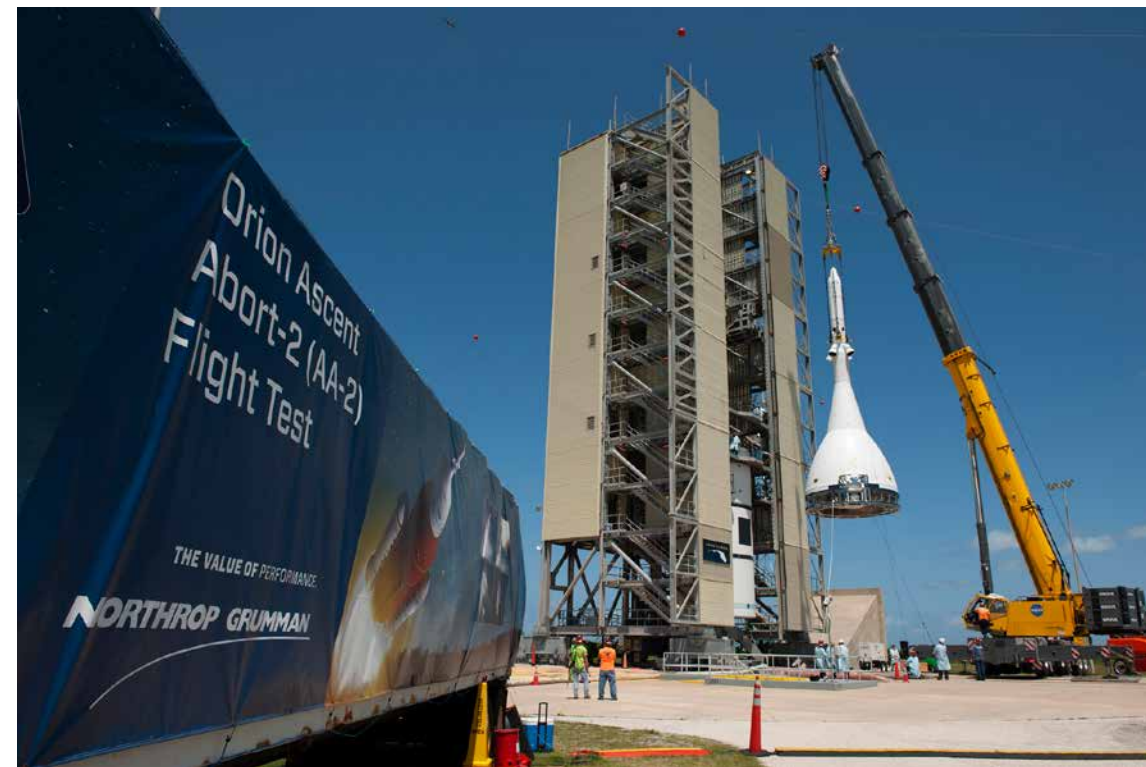
Above: A test version of the Orion crew module was integrated with the Launch Abort System on May 18, 2019. It was then lifted by crane for transfer to a KAMAG transporter. Photo credit: NASA/Glenn Benson
