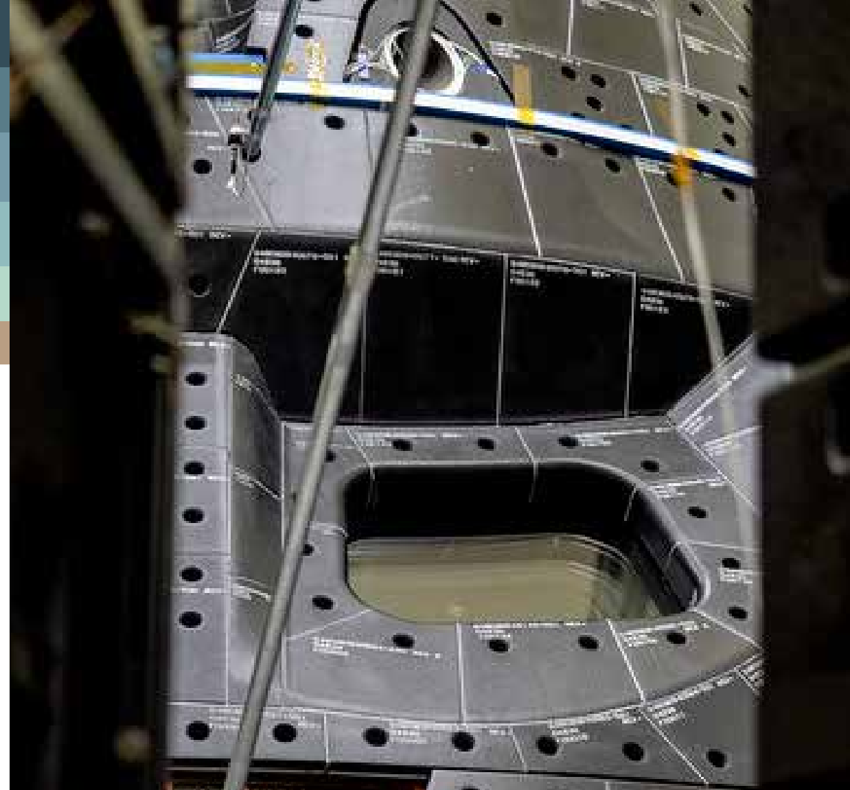
Left: The Orion crew module for Artemis 1 recently completed windows testing where engineers used a laser interferometer to determine — with extreme precision — the level of distortion and imperfection to ensure high quality optical performance. Photo credit: NASA/Rad Sinyak
