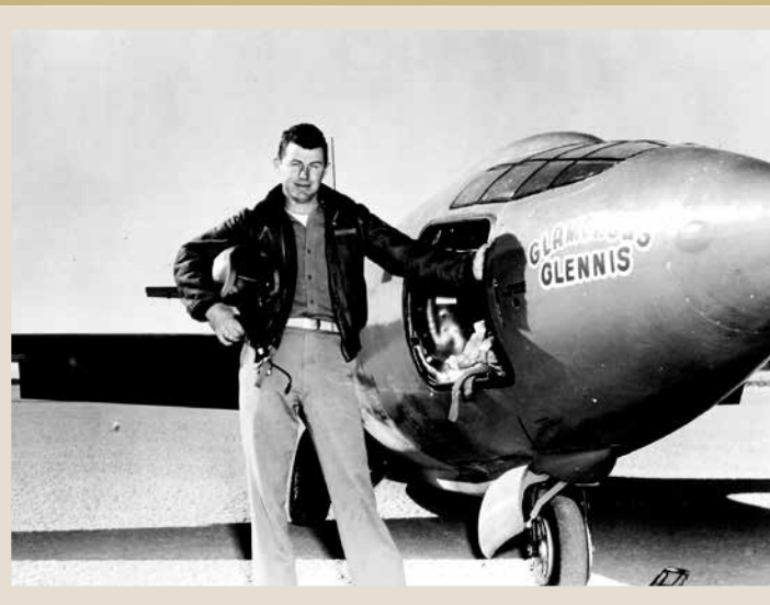
Chuck Yeager stands next to the rocket-powered X-1 aircraft. He broke the sound barrier on Oct. 14, 1947, flying the X-1 at Mach 1.06 (700 miles per hour or 1.06 times the speed of sound). He named the experimental plane Glamorous Glennis after his wife. Photo credit: U.S. Air Force
