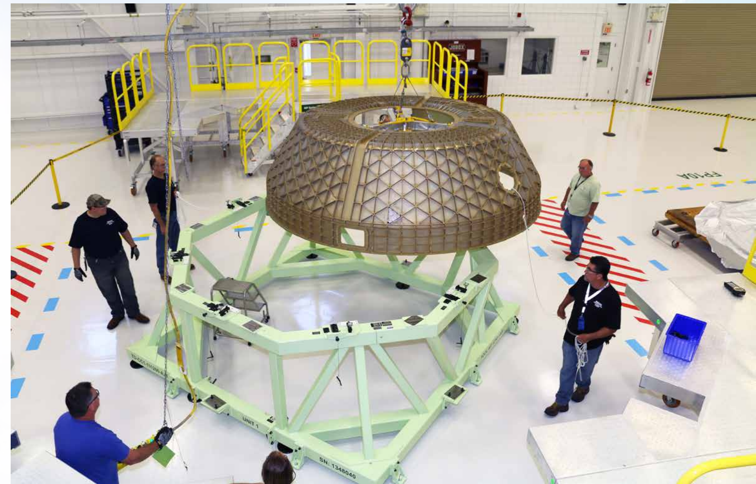
Engineers move the upper dome assembly of the CST-100 Starliner Structural Test Article onto a workstand inside the Commercial Crew and Cargo Processing Facility at NASA's Kennedy Space Center in Florida. Photo credit: Boeing
