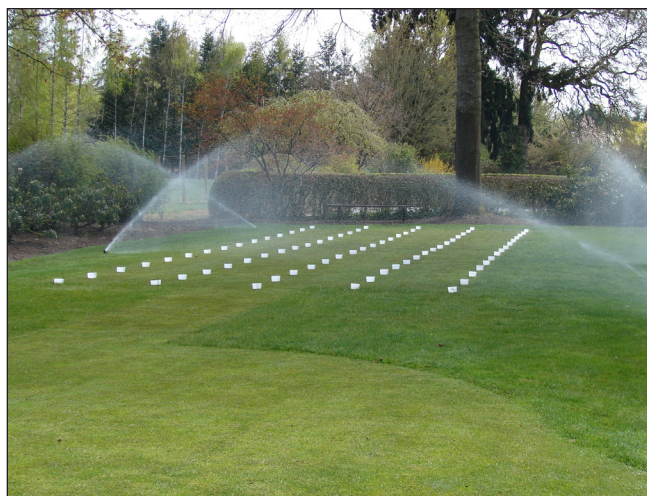
Figure 4. Catch cans can be used to evaluate the water delivery rate of a sprinkler system.
