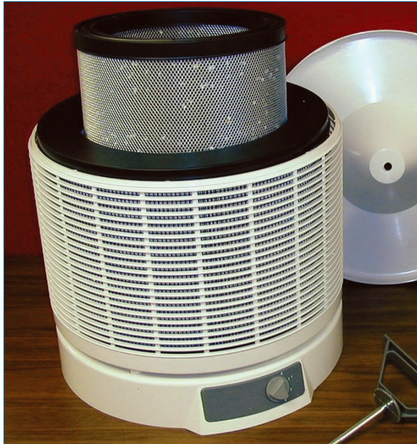
Figure 3-3 A tabletop recirculation filter unit with a substantial adsorber is a simple means of providing higher levels of CBR protection to unventilated safe rooms.
