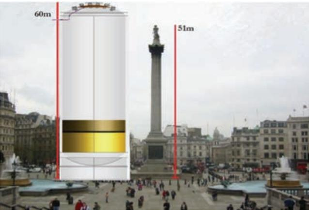
Storage cells are also an integral part of many of the concrete installations; the three Brent concrete structures have a total of 64 cells measuring 60m in height each - figure 2 opposite gives an indication of the scale of these cells.
