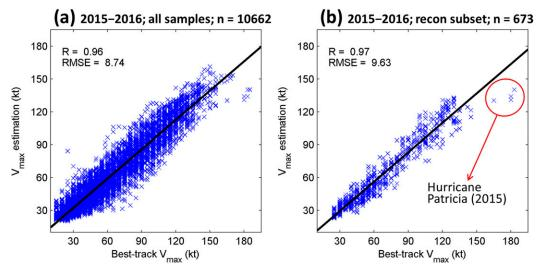
FIG. 11. (a) Scatterplot of CNN-TC estimations and best track intensities in the validation dataset of 188 global TCs in 2015–16. The sample number n, least squares regression line (black line), correlation coefficient R, and RMSE are also shown. (b) As in (a), except for samples with recon-aided best track for which aircraft reconnaissance observations were available within a  $\pm 3$ -h period.
