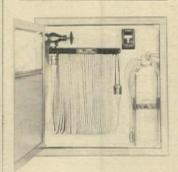
Shallow-wall cabinet. Fire extinguishers and hoses fit into cabinets that can be completely recessed in a 6" wall or semirecessed in a 4" wall. Cabinets accommodate a 10lb dry-chemical fire extinguisher, and can be used with or without a fire alarm. Frames are steel, aluminum, or stainless steel. Potter-Roemer, Inc., 2856 Leonis Blvd., Los Angeles, Calif.
