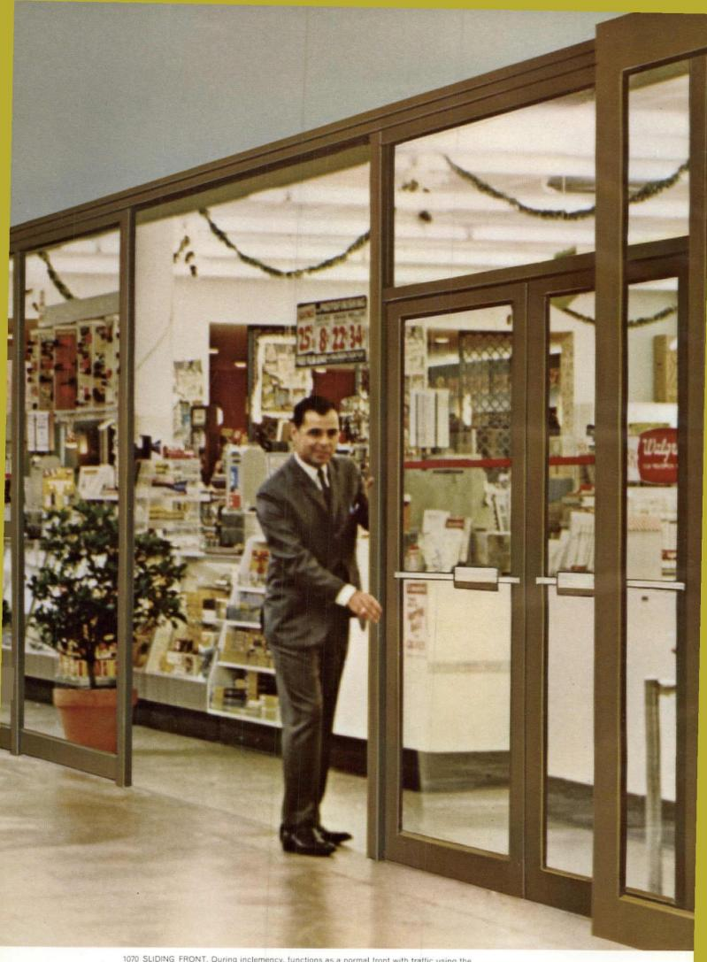
1070 SLIDING FRONT. During inclemency, functions as a normal front with traffic using the swinging doors. In fair weather—or in enclosed malls—the entire front rolls away. Glides on a single flat track set flush with floor. The Kawneer 1040 Sliding Front is similar, but without swinging doors. Panels can turn 90 degrees, permitting flexible storage arrangements.
