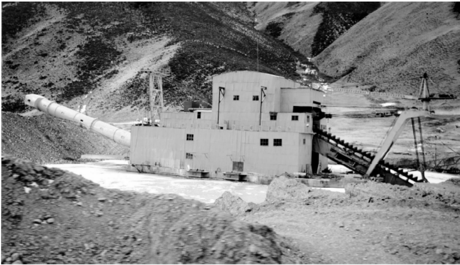
A floating dredge becomes frozen in a river in Lithang in mid-winter. These machines destroy fish habitats, muddy the water and alter stream beds in their quest for gold. Source: Tibet Outside TAR 1997, p 688.
