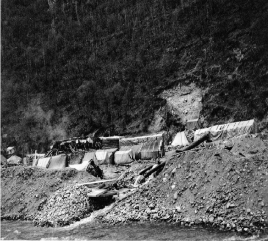
A typical small-scale Chinese gold rush camp that sluices alluvial placer gold from mountain streams. This camp is located in Karze in eastern Tibet, above Derge town, near the Cho-la Pass. Source: Tibet Outside TAR 1997, p 967.
