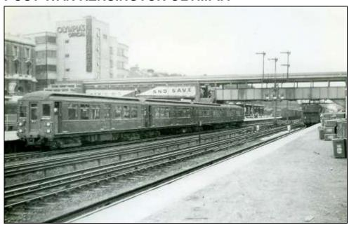
Left: A four-car train of District H Stock stands at Kensington Olympia, which comprises 1910-14 C, D and (at the rear) E Stock. Viewed from the up platform looking north, the train is standing at the south end of the Down platform, which was the limit District Line trains. although it was possible in an emergency for them to be shunted north of the station to cross over. To that end, all four tracks were once again electrified when District Line services began in 1946.
