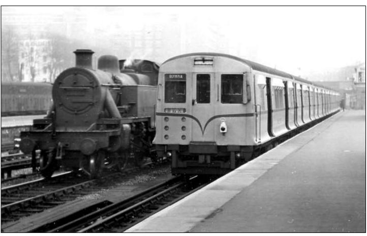
**Above:** The District Line's pride and joy in the mid-1950s was its train in unpainted aluminium, six out of the eight cars being seen in the Down platform. Note that there are no current rails on the through roads – these had been removed in 1956. In keeping with providing modern trains for a prestige service, the 1910-14 H Stock on this service was withdrawn as soon as possible.
