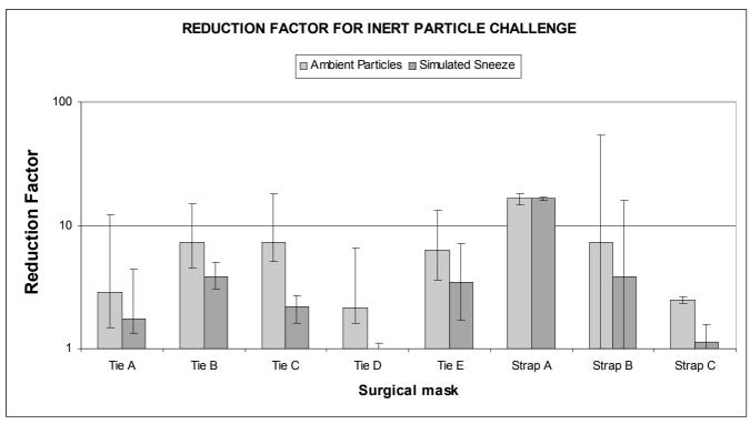
Figure 3.3. Inert particle reduction factors for all the surgical masks tested. Error bars show the spread of results measured
