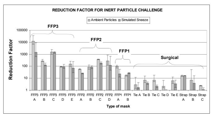
Figure 3.2. Inert particle reduction factors for all filtering facepieces and surgical masks tested. Error bars show the spread of results measured
