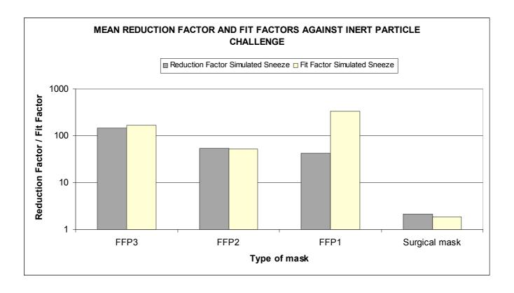
Figure 3.6 Mean values of the reduction factors and fit factor results for the grouped range of filtering facepieces and surgical masks tested against the inert simulated sneeze
