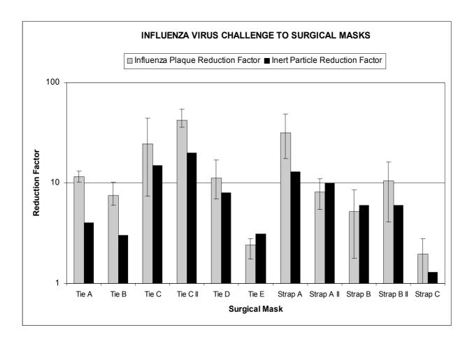
Figure 3.7. Mean (harmonic) influenza plaque reduction factors and associated inert particle reduction factors for all surgical masks tested. Error bars show spread of the calculated data
