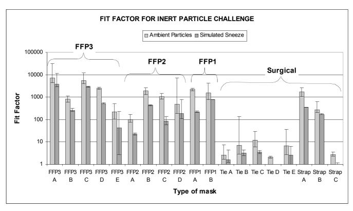
Figure 3.4. Fit factors for all filtering facepieces and surgical masks tested. Error bars show the spread of results measured
