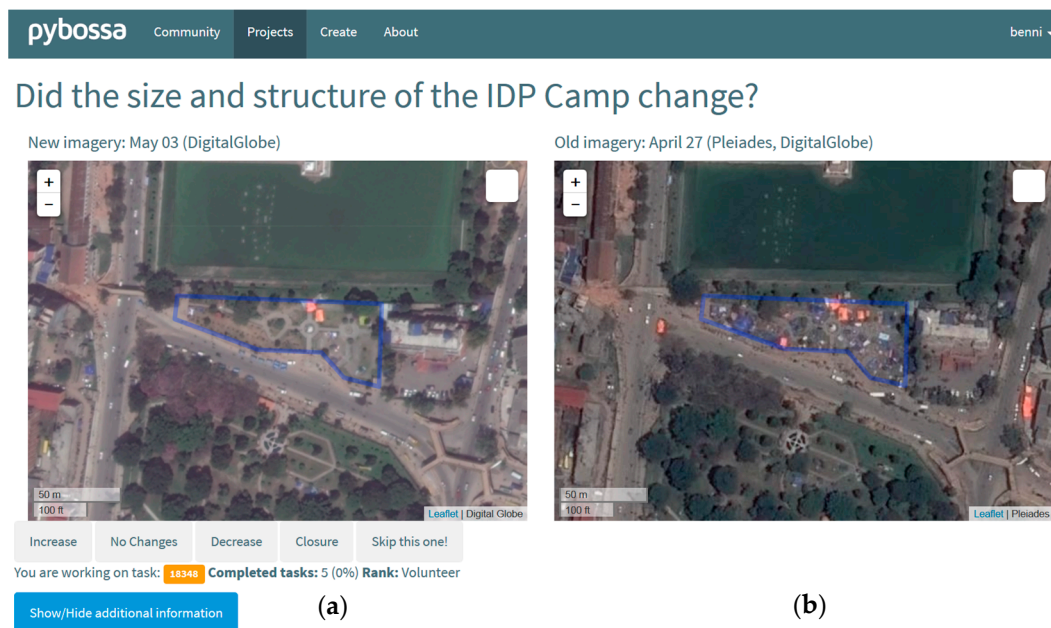
Figure 3. PyBossa crowdsourcing tool configured to present conflation tasks aimed at updating and validating shelters mapped after the 2015 Nepal Earthquake. On the (a) side of the image, a more recent image is shown, whereas on the (b) side, the reference image used for mapping is presented. The overlaid blue polygon is a mapped shelter object that comes from the OpenStreetMap database. Volunteers should analyse the three data sources to check if the shelters mapped before are still valid. Source: Anhorn et al. (2016) [23].
