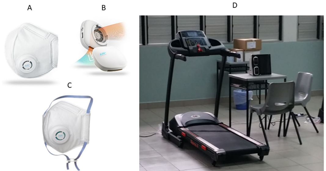
Figure 1. Illustration of the (A) disposable N95-class particulate respirator that is able to be paired with the (B) novel, reusable micro fan (C) AIR+ Smart Mask (D) Experimental set up.
