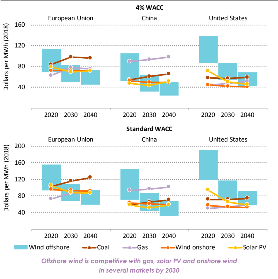
Figure 14.25 ▶ Evolution of offshore wind competitiveness: value-adjusted LCOEs by technology and region in the Stated Policies Scenario
