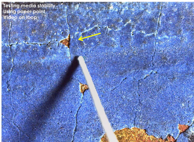
Fig. 13. Frame capture from a video of testing media for stability. Observing change in shadow profile as the chip is lightly touched with the paper point. 15 x. MS Typ 443. Houghton Library, Harvard University.
