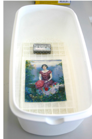
Fig. 23. When the gellan gum squares were removed, the paper and much of the adhesive was stuck to the gellan gum.
