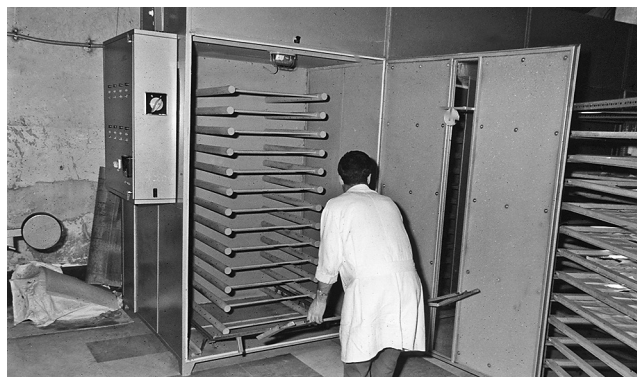
Fig. 27. A loaded trolley being pushed into a drying cabinet.
