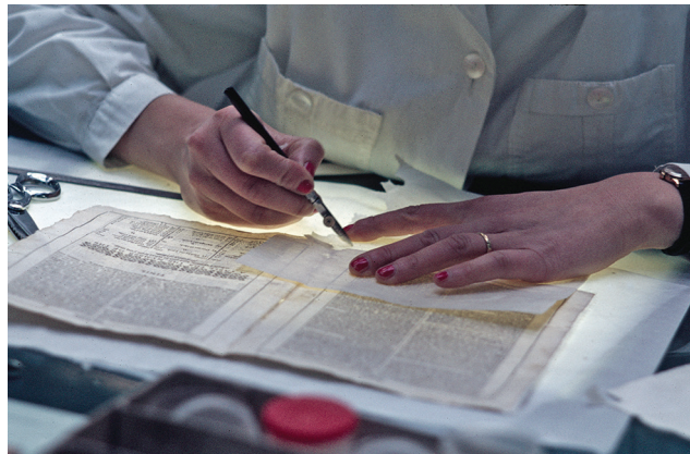
Fig. 30. Japanese tissue mending: cutting with a ruling pen.
