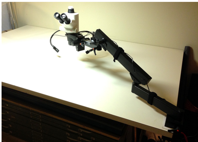
Fig. 3. Leica® S6D on a Unitron® Articulating (Flex Arm).
