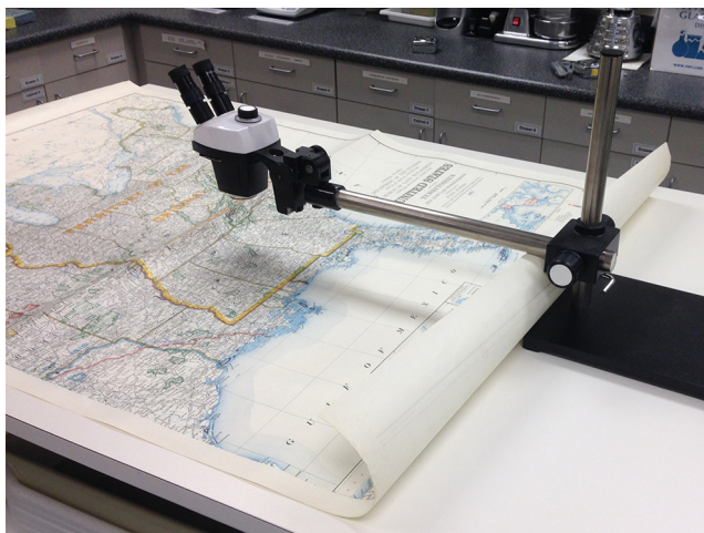
Fig. 2. Attempting to get a stereomicroscope, on a boom stand, into the middle of a large map. This required that the map be rolled at one end under the boom arm.
