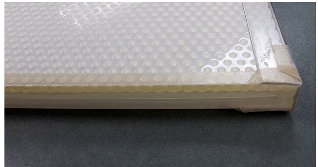
Fig. 23. Teflon tape is used to seal the two non-endcap sides of the platen.
