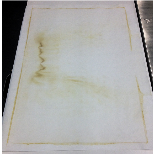
Fig. 7. TEK-Wipe on the suction table will draw more water than blotters or filter paper and prevent the formation of tide lines on artefacts.
