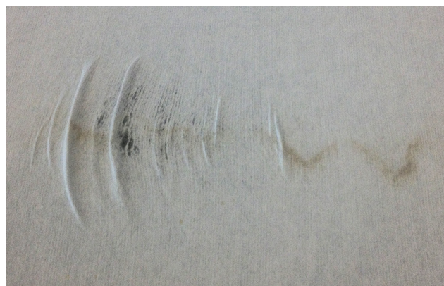
Fig. 3. Defibrillation occurring in TEK-Wipe from scrubbing.
