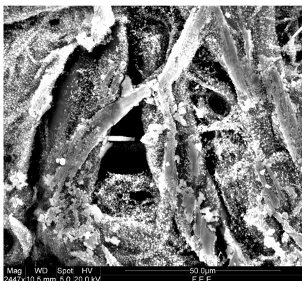
Fig. 5. Corroded iron deposit with fibers coated with corrosion: sample 2, immersion treatment with DTPA at 2447xM at 10.5mm working distance, area 2. Image taken by Kayleigh Fuller, Conservation Program staff.
