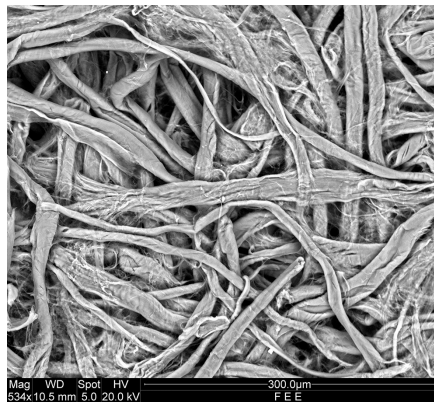
Fig. 3. Slightly hydrated and less compacted fibers: sample 2 immersion treatment in DTPA at 534xM, working distance 10.5mm, area 3. Image taken by Kayleigh Fuller, Conservation Program staff.
