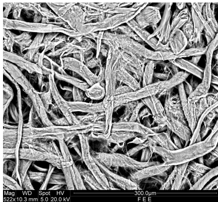
Fig. 2. Untreated, desiccated and compacted fibers: control at 522xM, working distance 10.3mm, area 1. Image taken by Kayleigh Fuller, Conservation Program staff.
