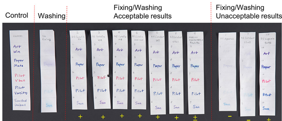
Fig. 4. After treatment. Five different pens applied on Whatman filter paper were locally fixed with 10 different fixatives mixed in methylcellulose A4M gel and then washed in a bath by immersion. The paper strips from left to right indicate control, washed without fixing, washed after fixing with Cartafix FF (+), Cartafix WA (+), Cartafix WE (+), Cassofix FRN-300 (+), Catiofast 269 (+), Catiofast 159(A) (+), a mixture of Mesitol NBS and Rewin EL (- and +), Appretan N 92100 (-), Catiofast 2345 (-), and Lupamin 9095 (+). The plus (+) and minus (-) signs below the paper strips indicate the ion charges of each fixative.
