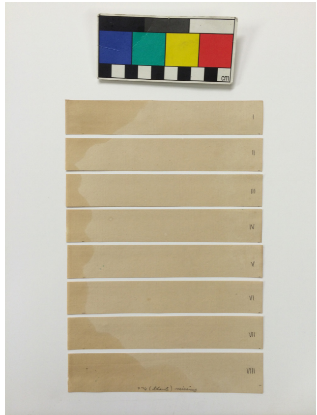
Fig. 2. End sheet cut into test strips for experimentation. Photograph by Scott Nolley.
