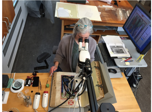
Fig. 3. The microscopy station as seen from above, including tools, consolidation supplies, the computer monitor displaying the treatment image of the illumination, and the notebook of treatment notes and records.
