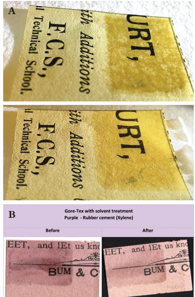
Fig. 10. (a) Visible reduction of surface adhesive on yellow masking tape after four 12-minute applications of Gore-Tex sandwich (xylene). (b) Before and after Gore-Tex and solvent treatment images of the purple rubber cement sample.
