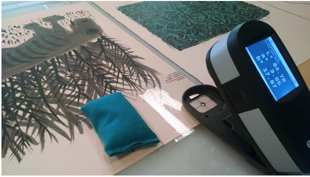
Fig. 15. The X-Rite eXact spectrophotometer set up for before treatment documentation of paper tone.
