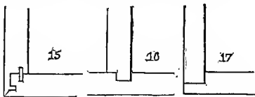
Modes of notching for boards are shewn in figs. 16, 17, and 18. Fig. 16 is called a nosing , also shewn at fig. 21, in its common application for fixing the risers to the treads of staircases. Common
