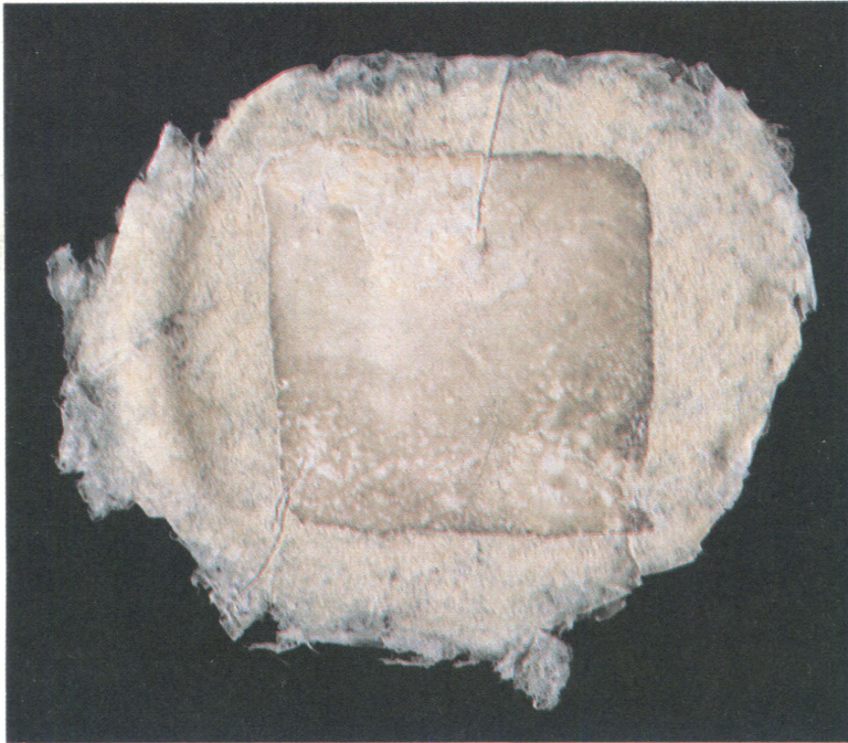
Color pl. 5. White lead sample on cast rag paper with a high alum content. After exposure to a hydrogen sulfide environment, pink appeared in the upper left corner of the paint square.
