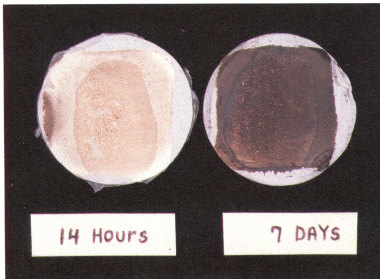
Color pl. 2. Two white lead samples marred with thumbprints. After fourteen hours, pink discoloration is visible beneath the thumbprint; after seven days, the thumbprint area has darkened with black lead sulfide.
