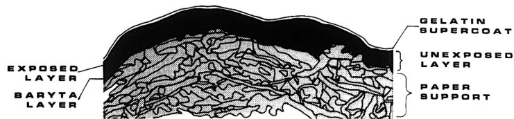
Fig. 6. Line drawing based on Figure 5. The various layers of this sample have moved over one another during cross sectioning and present a distorted view of the succession of the individual layers. The opaque band is the baryta layer coating the paper base to segregate the image-carrying gelatin layer from the paper fibers. The thin upper-most layer represents the gelatin binder and the silver image provides a grainy pattern toward the left side of the photomicrograph.
