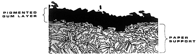
Fig. 2. Line drawing based on Figure 1. The pigment-bound layer is clearly visible as a dark surface sitting on and lightly penetrating the upper paper support
