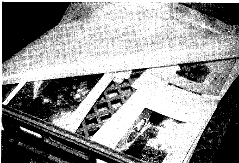
Albumen prints in final stages of air drying in bakery racks.
