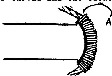
Fig. 27. Pack-sewn book before boards are drawn on. Sharp narrowing (exaggerated) at A gives thinner supports over the joints than would be the case for a comparable plain-sewn book; this allows a more flexible joint without excessive thinning of the support.
