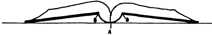
Fig. 8. "Self-closing" book. The spine is lined to be completely rigid; the joints (HB) are extremely flexible; the paper has good drapes.
