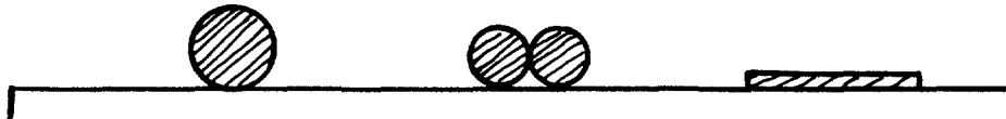
Fig. 12. Projection of sewing supports. The cross-section area of each support is the same. In this case the projection of the double cord is 4 times that of the tape (this ratio is not fixed) while that of the single cord is 1.4 times that of the double cord (this ratio is fixed).
