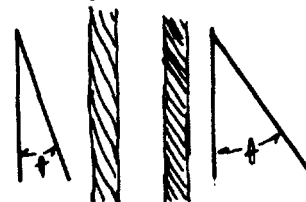
Fig. 19. Angle of twist. As the cord is twisted tighter, \theta grows larger; at the same time the cord gets shorter and more compact.
