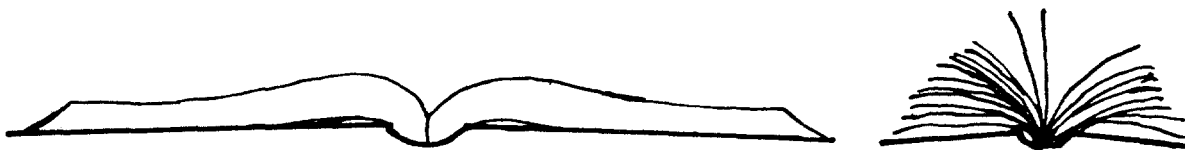
Fig. 1. Good and poor drape. Folio and duodecimo from the same paper; the 12mo is cross-grained as well as narrower.
