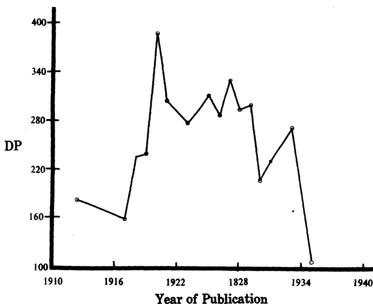
Figure 1. Degree of polymerization (DP) of various volumes of Chums (designated by Year of Publication).
