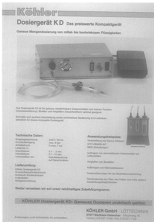
Fig. 8. Product literature describing the Dosiergerät KD made by Köhler GmbH, Germany
