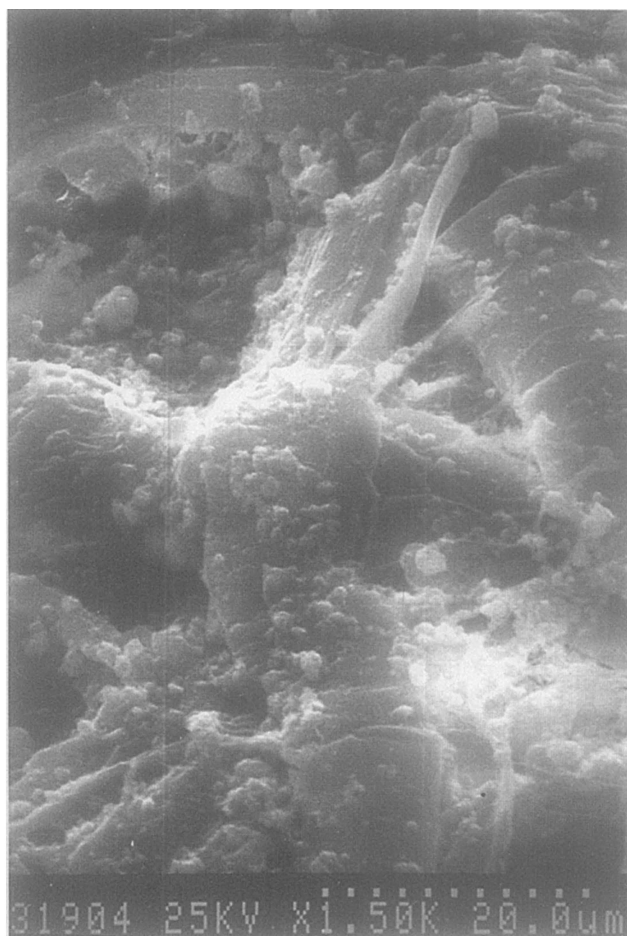
Fig. 5b. SEM photomicrograph of paper B, sample 3, treated side (1,500x). Magnesium containing particles are apparent on the treated side of the paper
