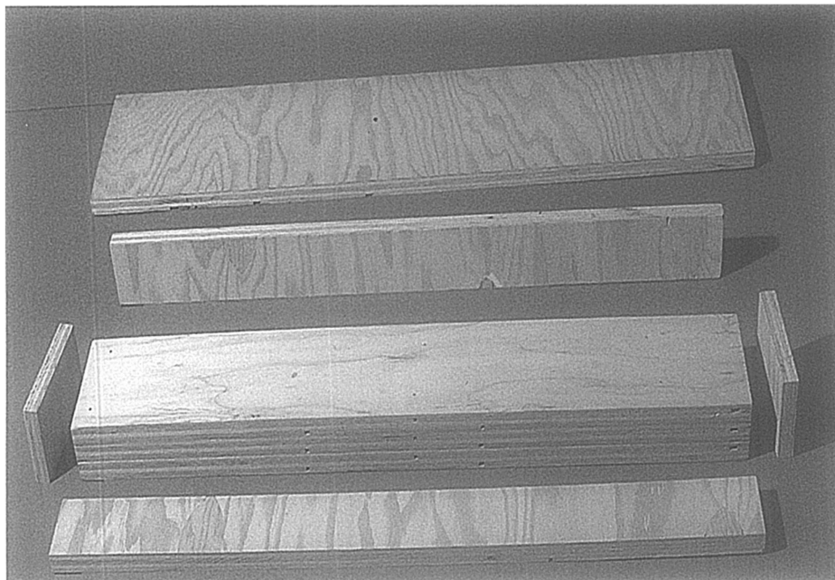
Fig. 8. Plywood mold for presentation box
