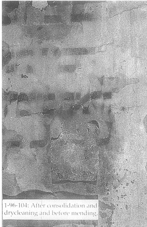
Fig. 10. Detail of verso of first sheet showing patch on loss shown in Fig. 9
