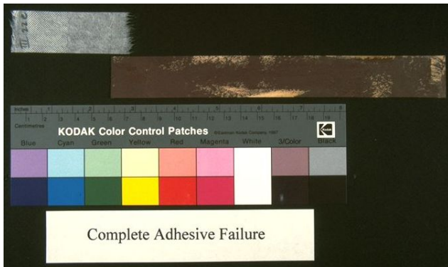
Fig. 9-10. Recto and verso of a sample # III.22.e. Full oil saturation corresponds with complete adhesive failure
