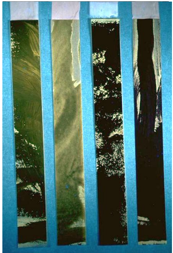
Fig. 15-16. UV/VIS Fluorescence. From left to right: Verso of samples I.13.d., II.20.d., III.22.c., IV.21.a. The more intense UV/VIS fluoresce reaction indicates that paint straight from the tube has a greater oil concentration than paint thinned with Winsor Newton oil painting medium
