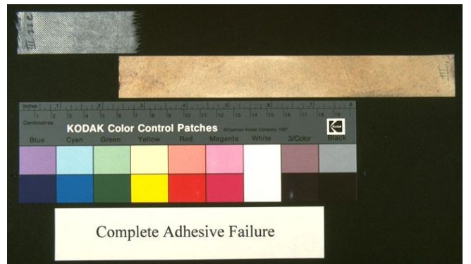
Fig. 9-10. Recto and verso of a sample # III.22.e. Full oil saturation corresponds with complete adhesive failure
