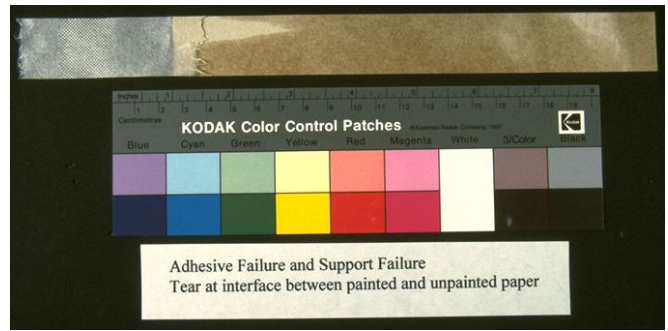
Fig. 7-8. Recto and verso of a variegated sample # II.20.d.. Failure occurring in the wheat starch bond corresponds directly to painted surfaces, and is discerned readily from intact bonds corresponding to unpainted surfaces
