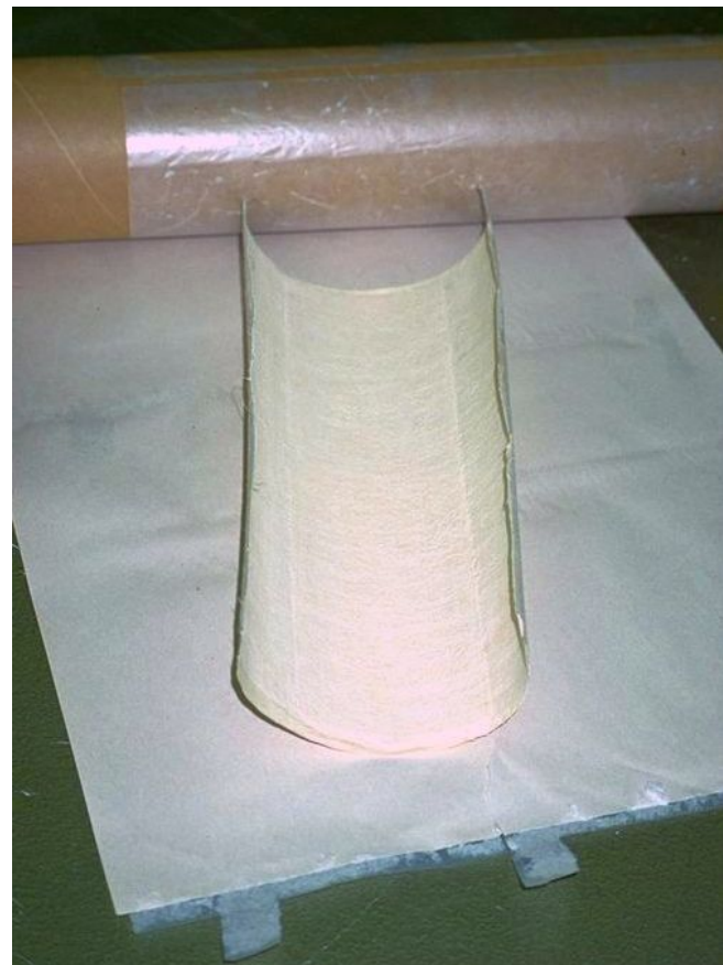
Fig. 19. Imparting a rounded shape to sewing support
