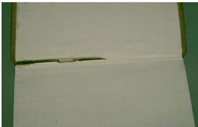
Fig. 32. Tear in endpaper joint
