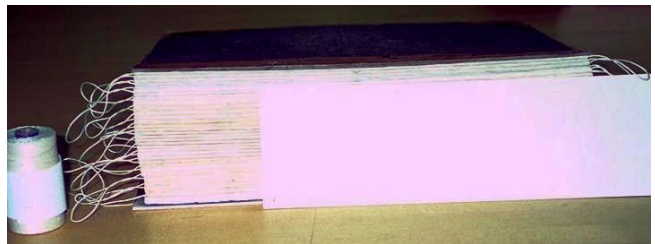
Fig. 21. Determining the natural spacing of the sewn gatherings
