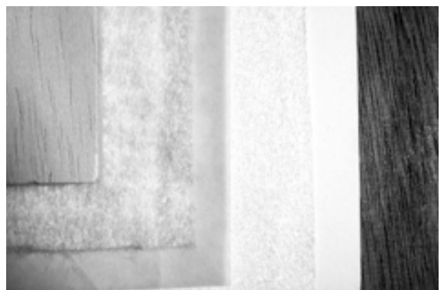
Fig. 8. Construction of the hard-soft sandwich.
