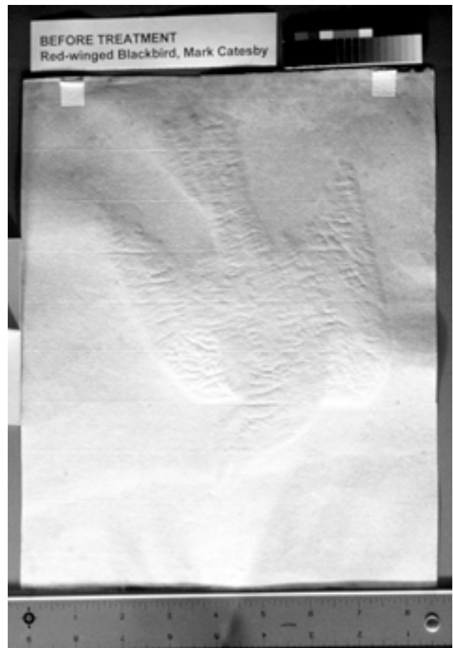
Fig. 2. Quilted distortion caused by varnish layer. Verso, raking light.
