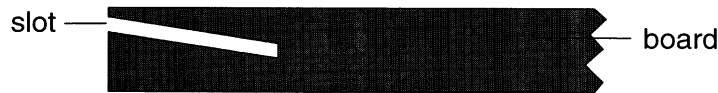
Fig. 3. Schematic diagram of a slotted board. The slot starts nearly directly underneath the leather and continues to the middle of the board's thickness. Its depth can vary between 5 and 8 mm.
