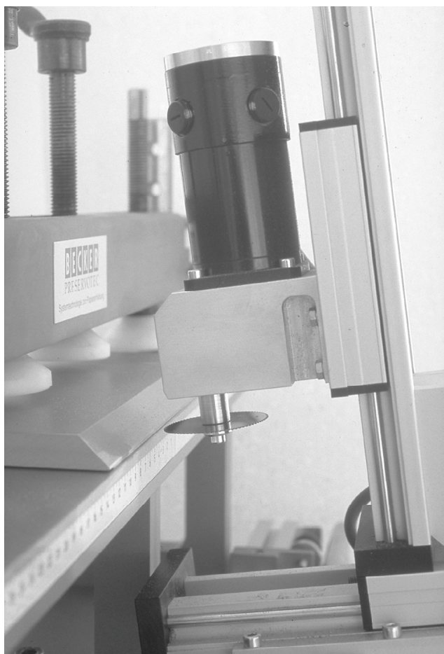
Fig. 6. The new board slotting machine: side view
